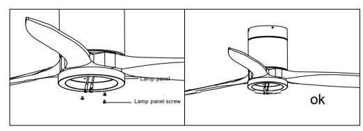
Unscrew a set screw. Attach the LED pan up to the bottom of the fan by inserting the other two set screw heads into key hole slots, rotate it to place, then secure the previous set screw by aligning screw hole and the hole at the bottom of the fan, tighten the rest two set screw to secure LED pan.
