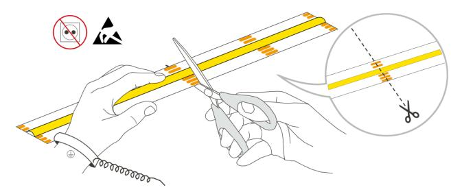
Calculate the needed length and cut off the extra length along the cutting mark if necessary.
