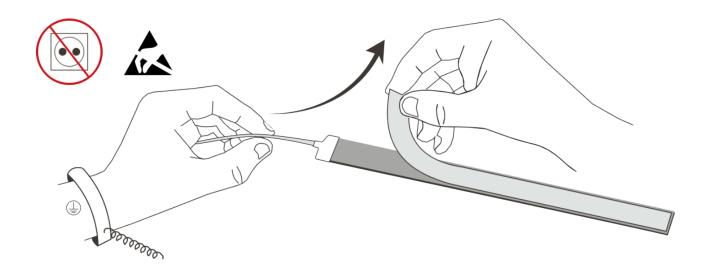
peel off the release paper of the tape ste p by step. Don't peel off all release paper at one time to avoid getting your strip in a mess.
