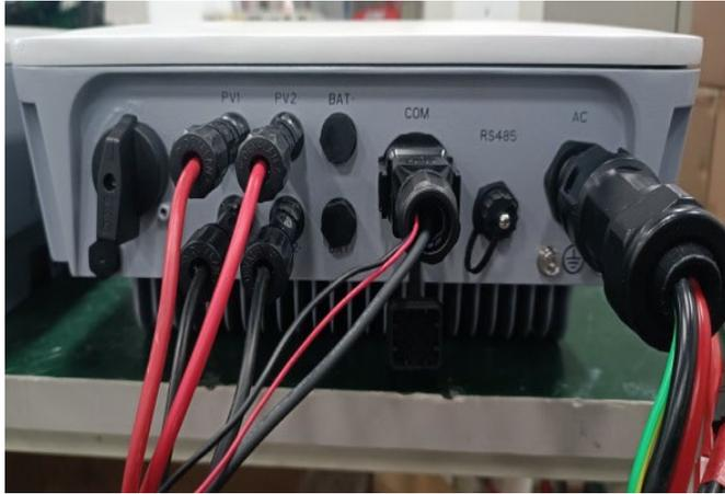
INV 2(Address 2): Only one RS485 signal cable is connected to INV1(not connected to the CT)
